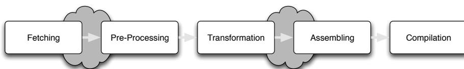
Figure 2.5: The presentation pipeline of ActiveMath: the content items are fetched from the content store on the far left and delivered within web-pages on the right.
